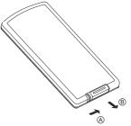
2. Replacing the battery Replace the battery with the same type and the (+) side facing up.
